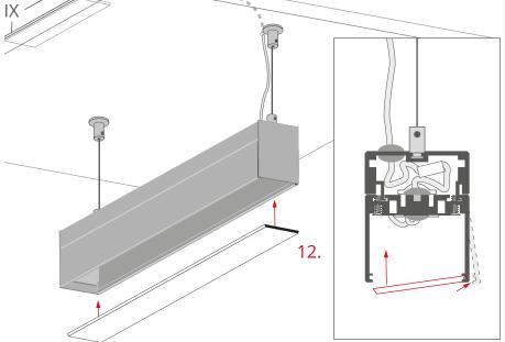
Attach the cover (12) by slightly bending the edge of the profile outwards.
