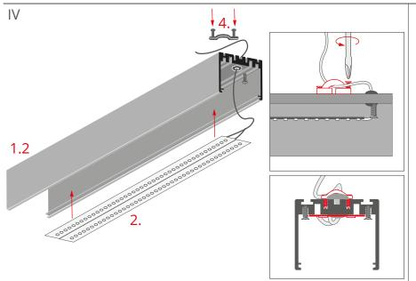
Adhere the LED tape (2) into the profile item (1.2). Run the power cable through the gland.
