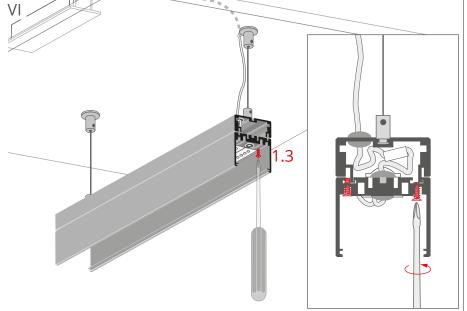
Secure the profile items against slipping out by tightening the locking bolts (1.3), embedded in the pre-drilled holes.
