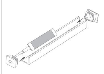
${\bf 3}_{\bullet}$  Apply a silicone layer to the bottom of the profile and embed the LED strip in it.
