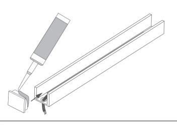
**OPTIONALLY:** Power cables can be run through the end caps in which case the extrusion does not need to be drilled through.
