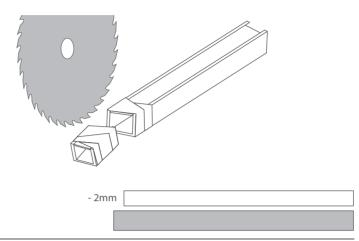
**NOTE!** Low precision cutting of the extrusion and cover can be done with a hand saw, however, uneven, jagged edges will remain, and the covers may break.
