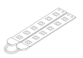
**OPTIONALLY:** The power cords can be led out from one pole of a given strip. This method is used to power suspended lighting fixtures.
