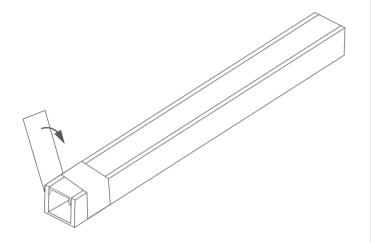
**2.** Use a mechanical saw to cut.
