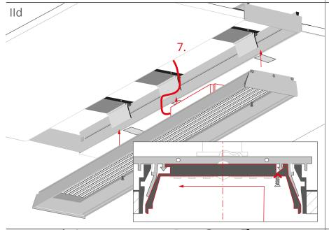
Connect the main power cables to the power supply (7).
