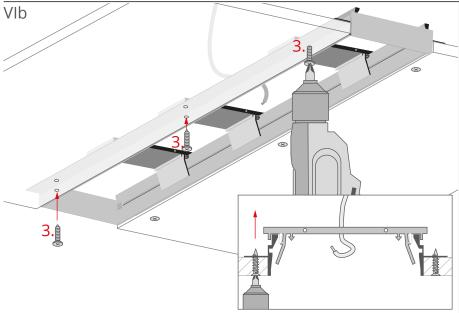
Insert the drywall screws (3) into the pre-drilled holes and tighten the second profile's flange to the drywall with them.
