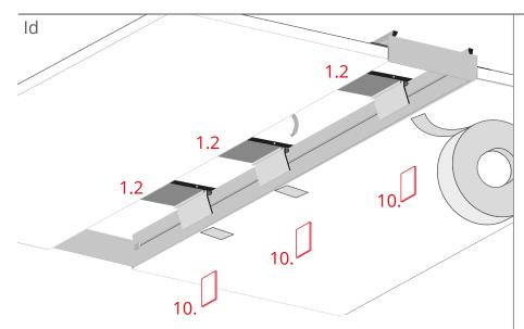
To facilitate further work, mark the location of the items (1.2) in the RAM-TEK-100 profile, e.g. with colored adhesive tape.
