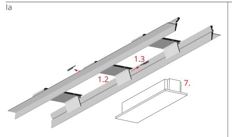
If the power supply (7) does not fit into the openings of the RAM-TEK-100 profile, its items (1.2) must be slid further apart accordingly.
