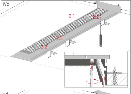
Secure the item (2.1) against slipping out by tightening the locking bolts (2.2) in the pre-drilled holes.
