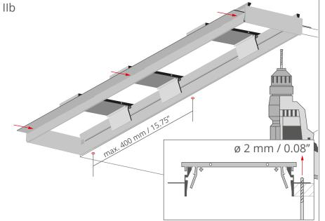
Put the profile to the edge of the drywall panel. Drill the holes through the panel and the profile's flange.
