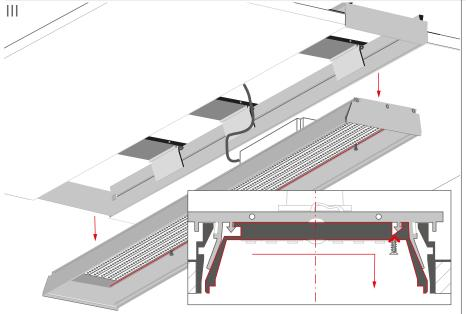
Slide the OMODO-100 profile towards the profiled orientation line and pull it down (as shown in the figure).
