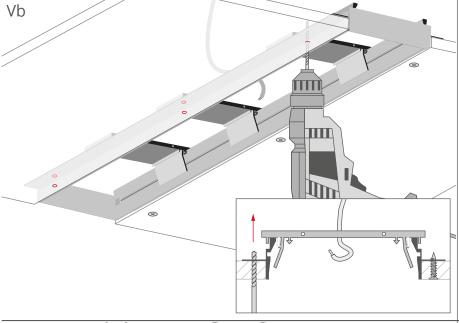
Drill the holes in the second panel and the profile's flange.
