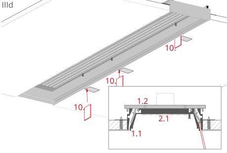
To prevent the OMODO-100 profile from falling out, insert wedges temporarily (10). They should be inserted into the marked spots in the gap between item (1.1) and item (2.1). There should be one wedge for each marked element (1.2) and they should be placed from the side of the profiled orientation line.
