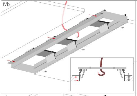
Place the second drywall against the profile. Lead the power cable through the openings in the profile.
