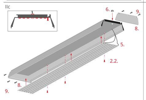
Adhere the LED tapes (5), mount the gland (6) and route the power cable through it.
