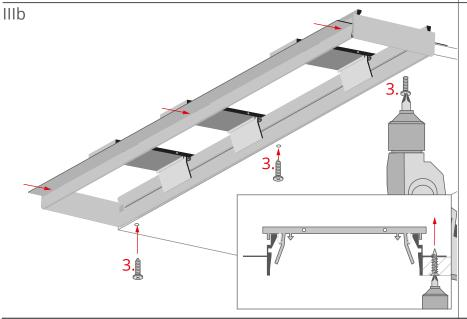
Insert the drywall screws (3) to pre-drilled holes and tighten the profile's flange to the drywall with them.
