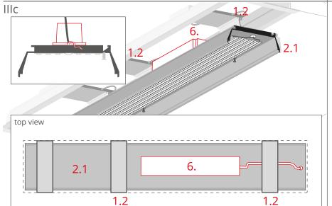
Mount the power supply (6) on the back of the profile in such a position that it fits into the opening of the RAM-KOL-100 profile.
