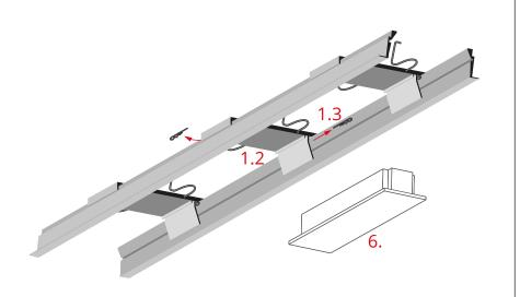
If the power supply (6) does not fit into the openings of the RAM-KOL-100 profile, its items (1.2) must be slid further apart accordingly.
