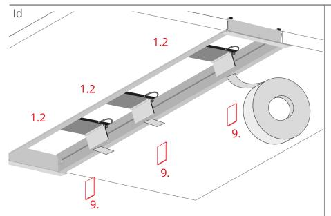
To facilitate further work, mark the location of the items (1.2) in the RAM-KOL-100 profile, e.g. with colored adhesive tape.
