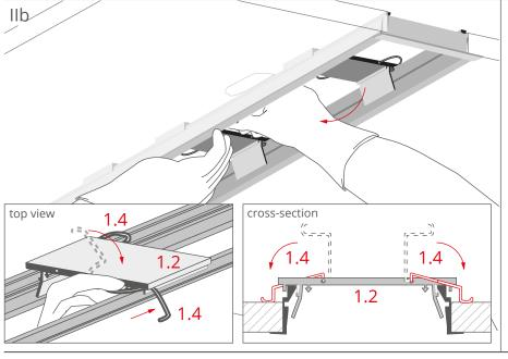
Lock the springs (1.4) at each item (1.2) by turning them, pressing them against the plate surface and sliding under the edge of the item (1.2) as shown in the figure.
