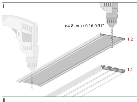
Drill holes with a diameter of 4-8 mm / 0.16-0.31" in the back of the mounting track (1.2). One hole per fastener.
