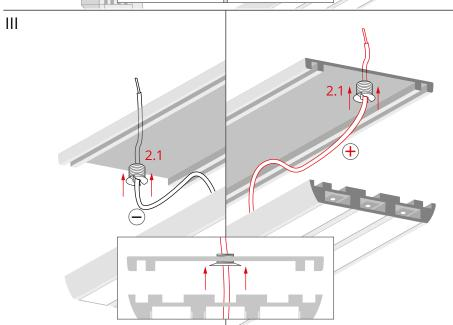
Insert the bolt (2.1) into the pre-drilled hole in the fixture. Run a cable from one pole of a LED strip through the bolt.
