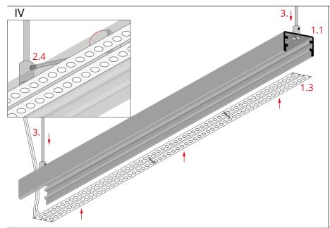
Mount and lock the rods (3), by tightening the pressure screws (2.4) in the heads of the fasteners.
