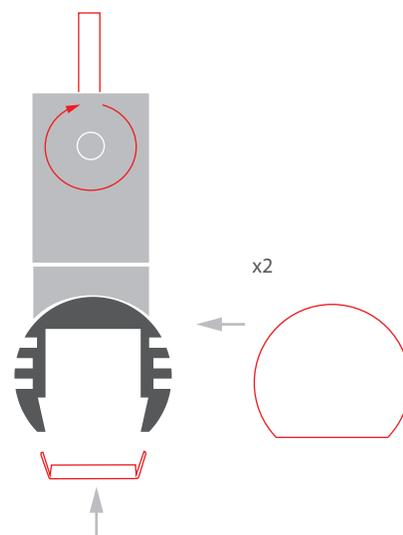
**5.** Install the W-KG ceiling fasteners. The fastener installation manual can be downloaded at [www.klusdesign.eu](http://www.klusdesign.eu). Place the power supplier next to the fastener and drill the ceiling to lead the cable to it.
