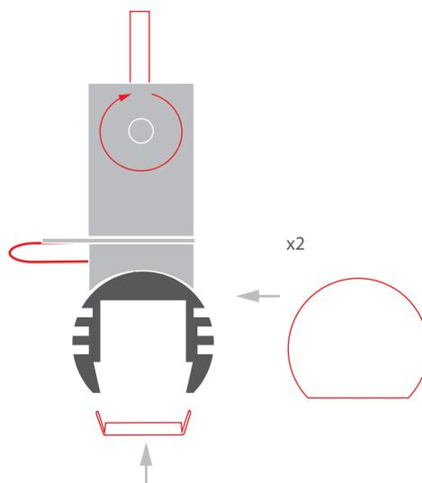
**5.** Install the W-KG-Z ceiling fasteners. The fastener installation manual can be downloaded at [www.klusdesign.eu](http://www.klusdesign.eu). Connect the cables, each for the single power pole to the fasteners. The cables should go through a pre-drilled hole just under the masking cover of the fastener.
