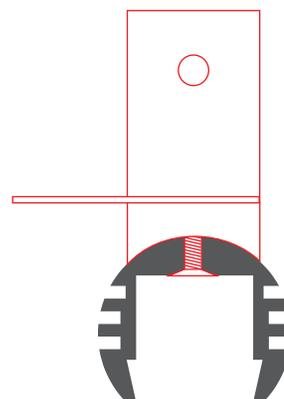
**3.** Mount the LED strip in the extrusion and lead the cables through pre-drilled smaller holes. Then lead them to the connector of the DP-ZZ-PDS-O fasteners. Each hole should lead a cable with one power pole, LED strip has to be cut before installation, so the wires can be easily routed to the holes.
