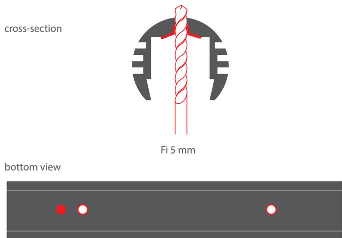
**2.** Mount the fasteners to the extrusion. Manual for the DP-PDS-O fastener can be downloaded from [www.klusdesign.eu](http://www.klusdesign.eu).
