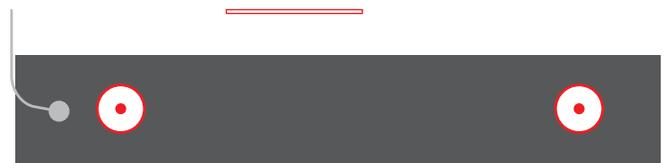
**5.** Install the W-KG ceiling fasteners. The fastener installation manual can be downloaded at [www.klusdesign.eu](http://www.klusdesign.eu). Place the power supplier next to the fastener and drill the ceiling to lead the cable to it.
