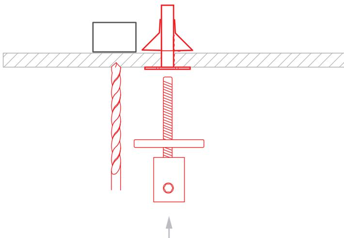
**6.** Mount the fixture with rods into the ceiling fasteners. Connect the cable to the power supplier, leading it through a pre-drilled hole in the ceiling.
