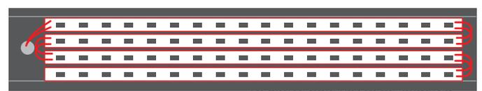
**3.** Install the PUSZ-LIN-LEB fasteners with rods on the mounting track and join the extrusion and mounting track with the use of BLOK springs. The fastener and 3035 installation manuals can be downloaded at [www.klusdesign.eu](http://www.klusdesign.eu).
