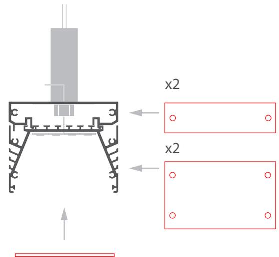
**5.** Install the W-KG-Z ceiling fasteners. The fastener installation manual can be downloaded at [www.klusdesign.eu](http://www.klusdesign.eu). Connect the cables, each for the single power pole to the fasteners. The cables should go through a pre-drilled hole just under the masking cover of the fastener.
