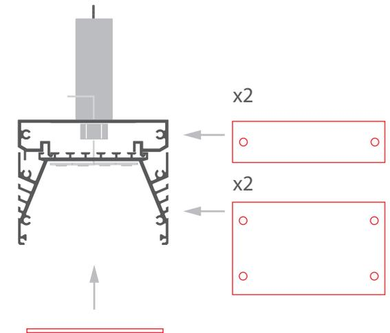
**5.** Install the W-KG-Z ceiling fasteners. The fastener installation manual can be downloaded at [www.klusdesign.eu](http://www.klusdesign.eu). Connect the cables, each for the single power pole to the fasteners. The cables should go through a pre-drilled hole just under the masking cover of the fastener.
