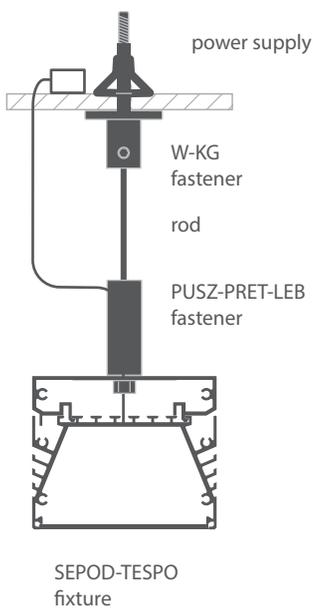
2) Rod - conductive driven power supply
