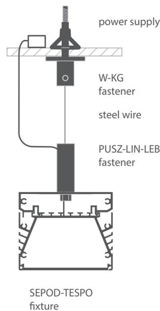
4) Wire - Rod - conductive driven power supply
