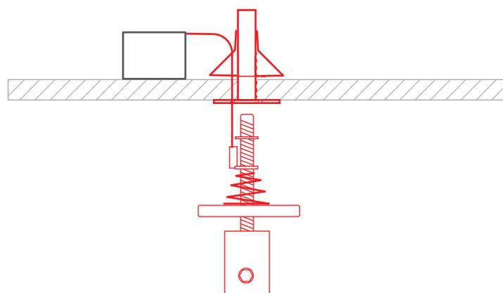
**6.** Mount the fixture with rods into the ceiling fasteners. Connect the cable to the power supplier, leading it through a pre-drilled hole in the ceiling.
