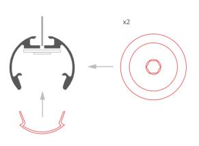
**4.** Insert the rods into the holes in the head of the conductive end caps in tighten them with an allen wrench.
