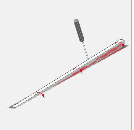
Using e.g. a flat screwdriver, pry up the fixture and remove it from the track.
