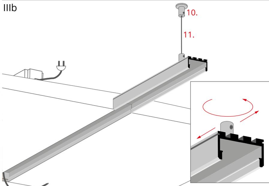
Connect the ceiling fastener (10) and the profile fastener with the wire (11).
