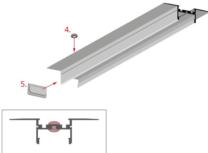
Attach the end cap (5) to the profile and install the gland (4) in the pre-drilled hole.
