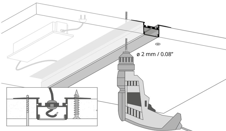
Drill holes in the second board and the profile's flange.
