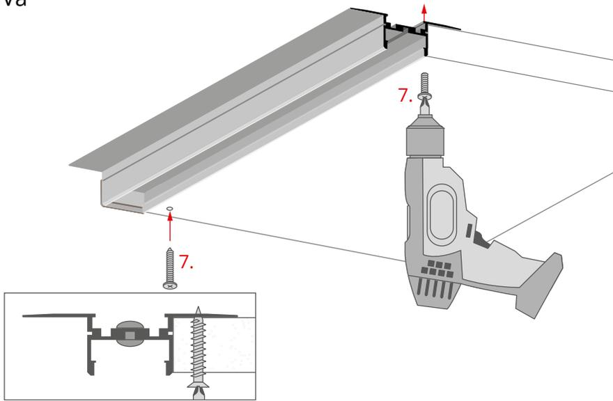
Insert the drywall screws (7) in the pre-drilled holes and screw the profile flange to the board.
