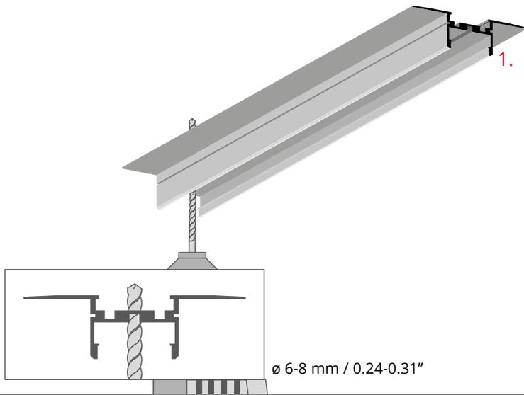
Drill a hole for the power cable in the GIZA-LL-UST (1) profile.
