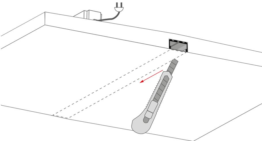
Cut layers of paint and plaster at the junction of the aluminum edge of the profile and the protective insert.
