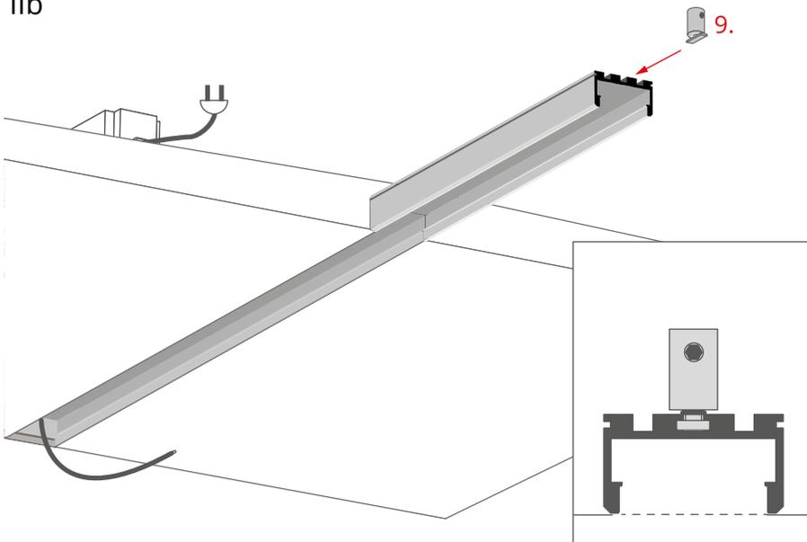
Insert the fastener (9) into the top channel of the profile.
