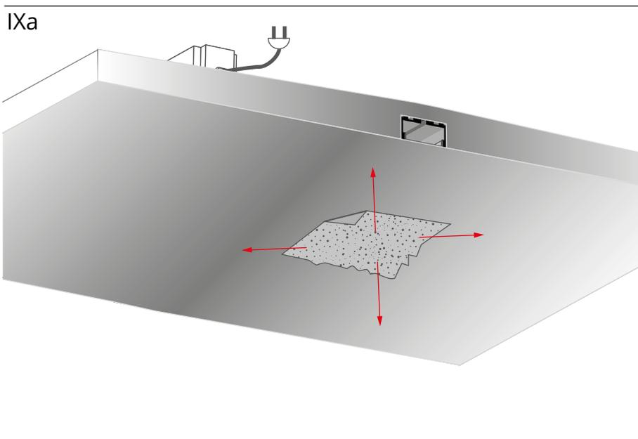
After the plaster has dried, sand the surface with sandpaper.
