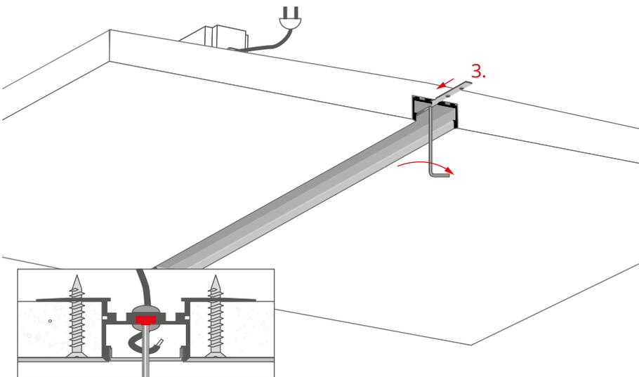
Insert the connector (3) into the channel inside the profile and tighten the locking bolts with an Allen key.
