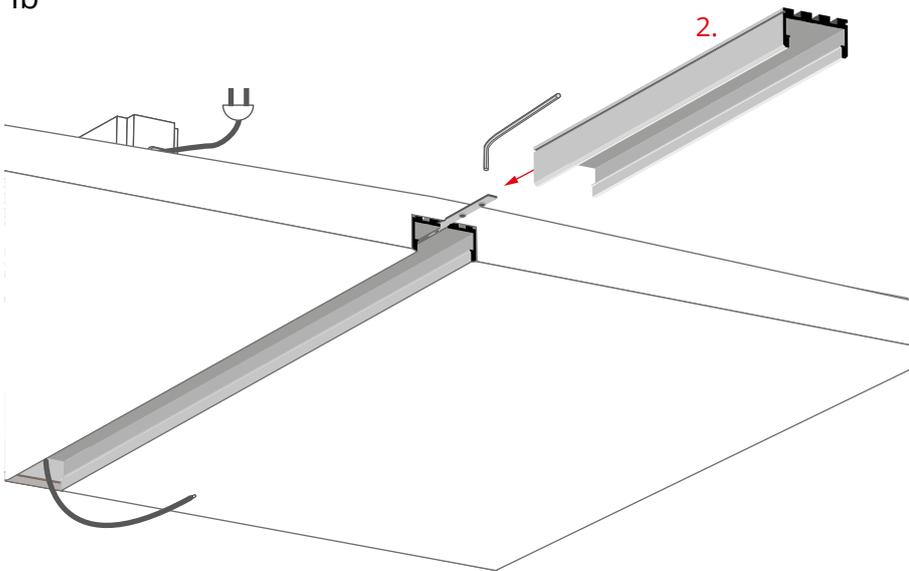
Slide the internal channel of the GIZA-LL profile (2) onto the protruding part of the connector. Finally tighten the connector screws with the Allen key.
