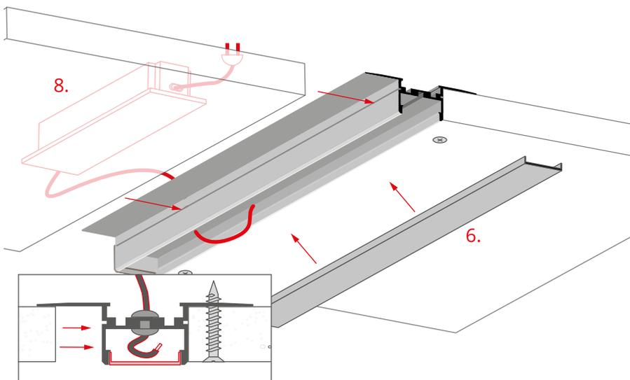
Route the cable from the power supply (8) through the gland.
