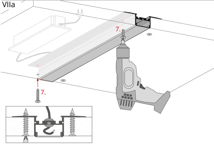
Insert the drywall screws (7) in the newly drilled holes and screw the second flange of the profile to the board.
