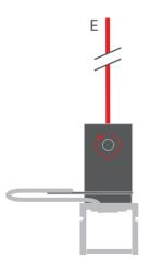
**12.** Attach the light fixture with the arm (E) to the top head (F). Block the rod by tightening the pressure screw in the top head with the Allen wrench.
