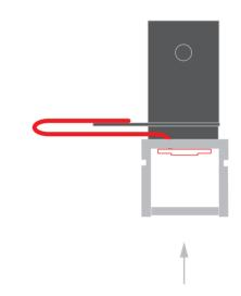
**11.** Insert the arm (E) into the mounting bracket of the head. Block the arm by tightening the pressure screw in the head with the Allen wrench.
